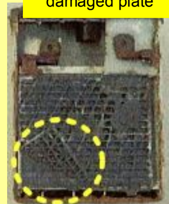
Example of damaged plate
